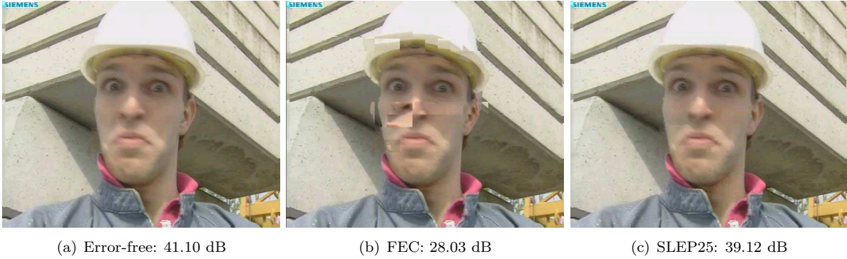
Fig. 7. Decoded frames from the Foreman sequence at a symbol error probability of 10^{-4} . 100 kbps of FEC fails to correct the channel errors, reducing the picture quality. At the same bit-rate, SLEP replaces the lost portions by their Wyner-Ziv decoded redundant counterparts and ensures acceptable picture quality. The 2 dB difference between the error-free picture and the picture decoded by SLEP is due to the quantization mismatch from Wyner-Ziv decoding.
