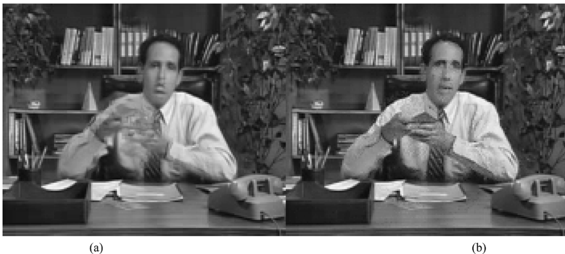
Fig. 8. Sample frame from QCIF Salesman sequence. (a) Decoder side information generated by motion-compensated interpolation. (b) Reconstructed frame after Wyner-Ziv decoding. Note that motion-compensated interpolation gives good results for most of the image. The localized large interpolation errors are corrected by the Wyner-Ziv bit stream.
