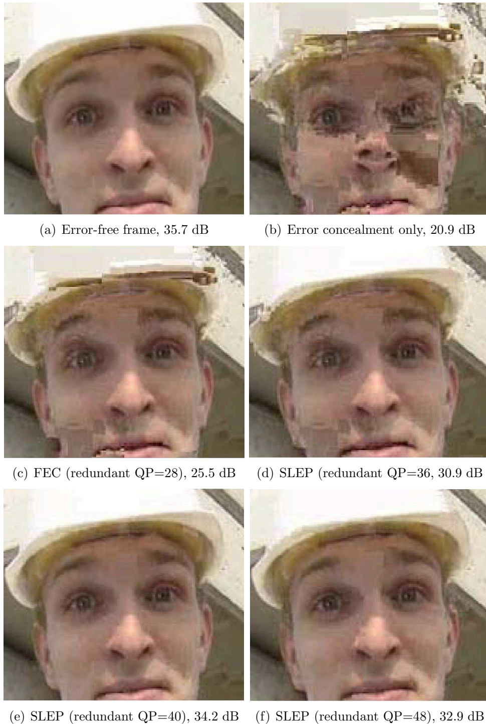
Figure 4.8: Cut-outs of a video frame from the Foreman CIF sequence. The primary description is encoded at 408 kb/s, while the error resilience bit rate is fixed at 40 kb/s. Robustness increases with the quantization step in the redundant slice (See fig. 4.2). However, with QP=48, the increased quantization mismatch reduces the decoded picture quality.
