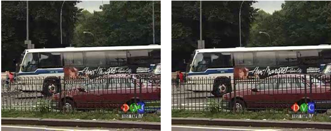
Figure 4.13: Decoded frames of the Bus CIF sequence encoded at 1024 kb/s, when the parity bit rate is 10% of the primary source coding bit rate. With FEC (left), decoding fails for some portions of the frame, reducing the PSNR to 20.2 dB. With SLEP scheme for a redundant description encoded at 25% of the primary bit rate (right), successful Wyner-Ziv decoding results in a PSNR of 30.3 dB, much closer to the error-free PSNR of 32.2 dB.
