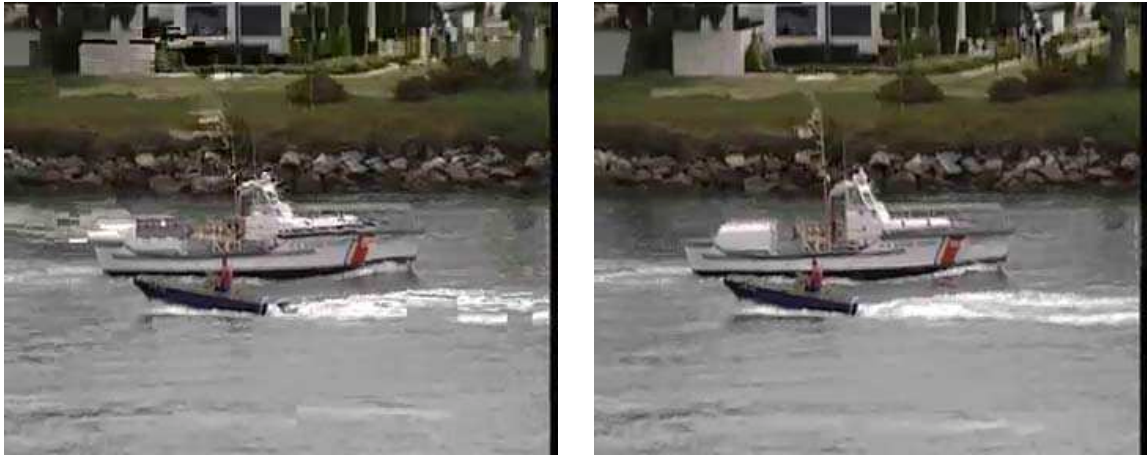
Figure 4.15: Decoded frames of the Coastguard CIF sequence encoded at 512 kb/s, when the parity bit rate is 10% of the primary source coding bit rate. With FEC (left), decoding fails for some portions of the frame, reducing the PSNR to 22.7 dB. With SLEP scheme for a redundant description encoded at 25% of the primary bit rate (right), successful Wyner-Ziv decoding results in a PSNR of 31.2 dB, much closer to the error-free PSNR of 32.9 dB.
