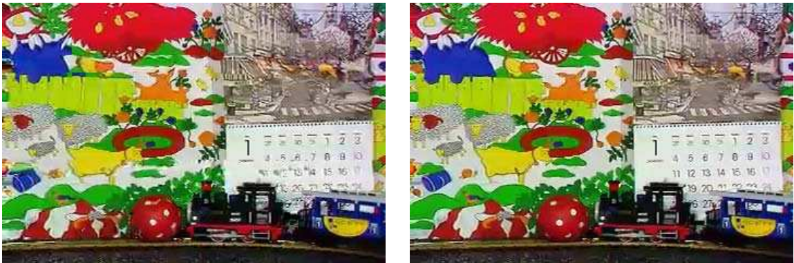
Figure 4.14: Decoded frames of the Mobile SIF sequence encoded at 768 kb/s, when the parity bit rate is 10% of the primary source coding bit rate. With FEC (left), decoding fails for some portions of the frame, reducing the PSNR to 17.3 dB. With SLEP scheme for a redundant description encoded at 25% of the primary bit rate (right), successful Wyner-Ziv decoding results in a PSNR of 25.3 dB, close to the error-free PSNR of 25.9 dB.
