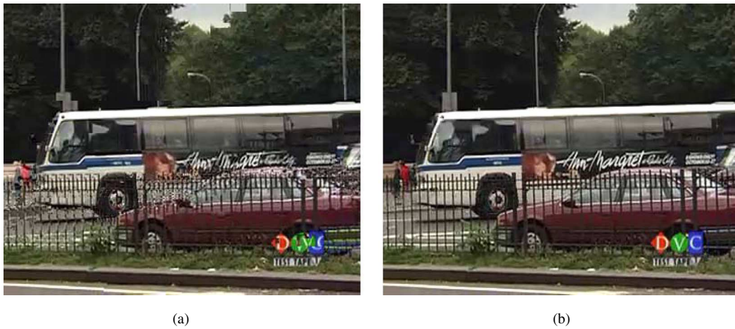
Fig. 9. Decoded frames of the Bus CIF sequence encoded at 1024 kb/s, when the parity bit rate is 10% of the primary source coding bit rate. (a) With FEC, decoding fails for some portions of the frame, reducing the frame PSNR to 20.2 dB. (b) With SLEP scheme for a redundant description encoded at 25% of the primary bit rate, successful Wyner–Ziv decoding results in a frame PSNR of 30.3 dB, much closer to the error-free PSNR of 32.2 dB.
